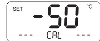
When replacing the heating element or the handle, the temperature if not accurate, can be calibrated by changing the following parameter.
